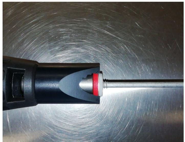
**Fig. 2** Example of a depth-locating nose piece with tapered sides
