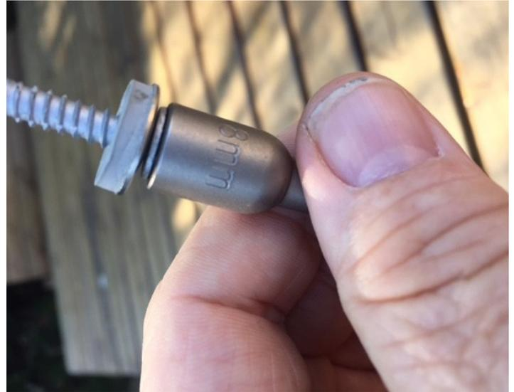
**Fig. 3** The socket must be deep enough so that the drive is on the flange at the base of the fastener head
